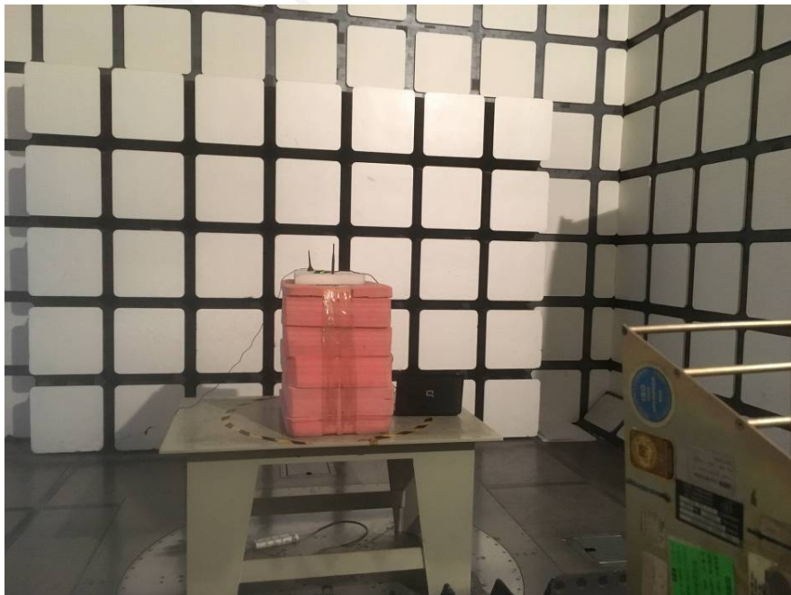
Radiated Spurious Emissions Test View (Above 1GHz)
